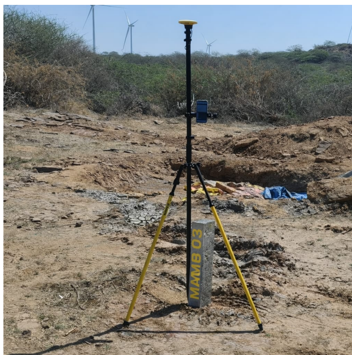
Photo-11.1: DGPS survey in the block using DGPS (Trimble GNSS)
