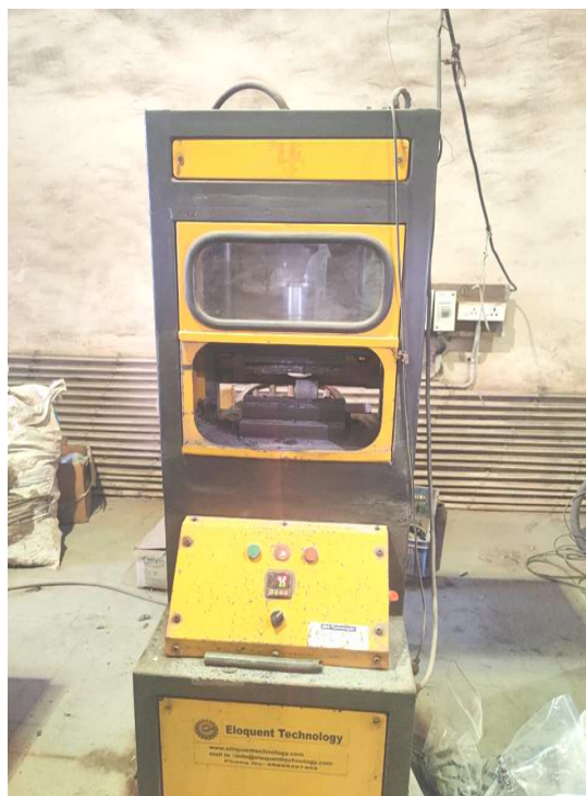
Photo-14.1: Photograph showing core splitter used to split borehole cores
