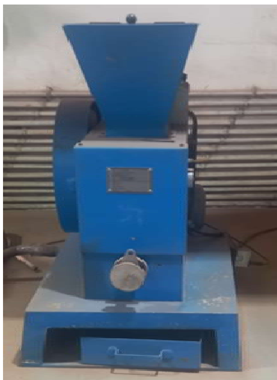
Photo-12.1 Photograph showing sample crusher used in sample processing
